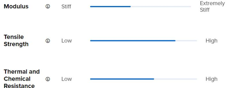
**Rigid 4000 Resin** Reinforced with glass for very high stiffness and a polished finish, highly resistant to deformation over time. Great for printing thin walls and features. Not suited for parts that must bend. Glass-filled Rigid 4000 Resin prints with a smooth, polished finish and is ideal for stiff and strong parts that can withstand minimal deflection. Consider Rigid 4000 Resin for general load-bearing applications.
