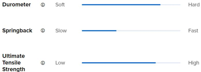
**Flexible 80A Resin** Simulates 80A durometer rubber, high impact resistance and compression, great for ergonomic soft-touch grips. Flexible 80A Resin is the stiffest soft-touch material in our library of Flexible and Elastic Resins, with an 80A Shore durometer to simulate the flexibility of rubber or TPU. Balancing softness with strength, Flexible 80A Resin can withstand bending, flexing, and compression, even through repeated cycles.
