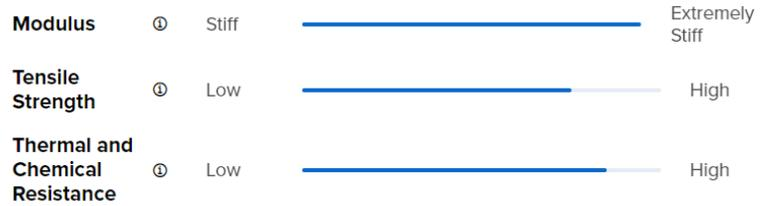
**Rigid 10K Resin** With a stiffness simulating that of glass and fiber-filled thermoplastics, Rigid 10K Resin is designed to maintain structural integrity under any condition. This highly glass-filled resin is the stiffest material in our engineering portfolio. Choose Rigid 10K Resin for precise industrial parts that need to withstand significant load without bending. Rigid 10K Resin exhibits a smooth matte finish and is highly resistant to heat and chemicals.
