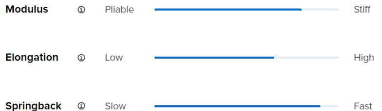
**Tough 2000 Resin** Simulates ABS plastic. Choose for applications that will undergo high stress and strain. Great for functional prototyping of assemblies, machining, and snap-fits. Tough 2000 Resin is the strongest and stiffest material in our functional family of Tough and Durable Resins. Choose Tough 2000 Resin for prototyping strong and sturdy parts that should not bend easily.
