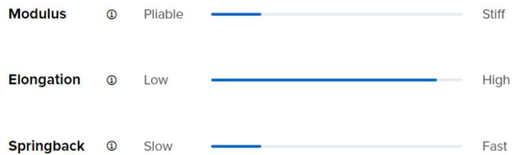
**Durable Resin** Similar physical properties to polypropylene (PP) or high-density polyethylene (HDPE), where high elongation, deformation, or impact resistance are required. Durable Resin is the most pliable, impact resistant, and lubricious material in our functional family of Tough and Durable Resins. Choose Durable Resin for squeezable parts and low-friction assemblies.
