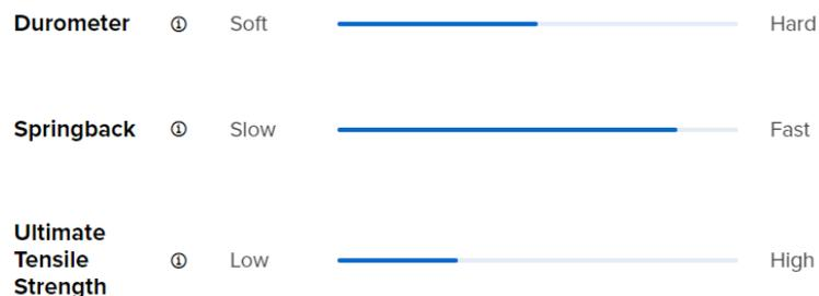
**Elastic 50A Resin** Designed for applications requiring high elongation and high energy return. Use for prototypes that must bend, stretch, compress, and hold up to repeated cycles. Our softest Engineering Resin, this 50A Shore durometer material is suitable for prototyping parts normally produced with silicone. Choose Elastic 50A Resin for parts that will bend, stretch, compress, and hold up to repeated cycles without tearing, and spring back quickly to their original shape.
